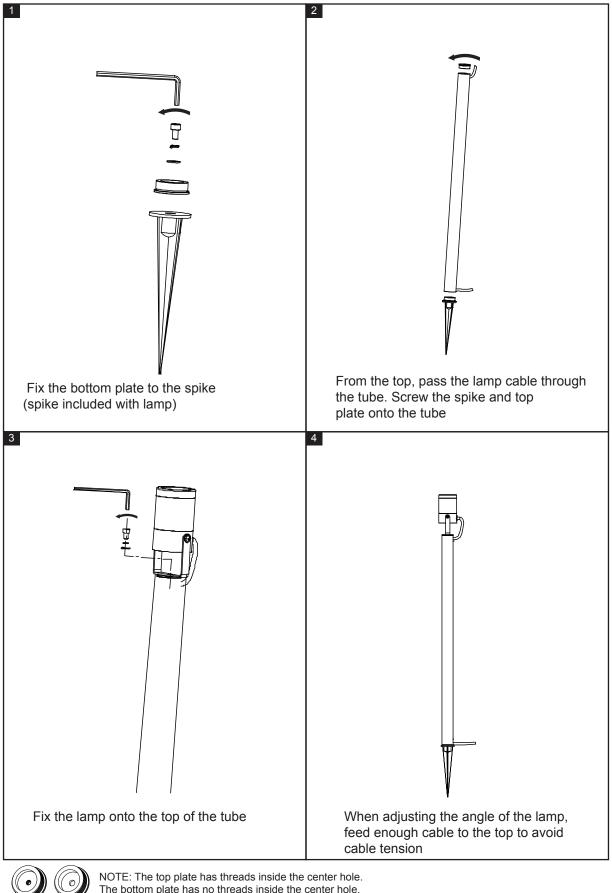
The bottom plate has no threads inside the center hole.
