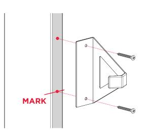
Mark holes through rack mounting plate, drill 1/8" pilot holes and install screws into stud. Tighten screws firmly.
