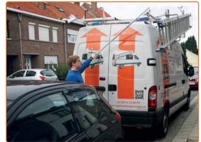
Handling from the sides makes (un)loading of ladders possible in confined parking spaces
