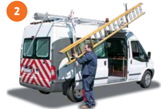
2 - Lift the rear end of the ladder onto the second support;
