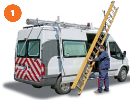
1 - Put the ladder on the front support;
