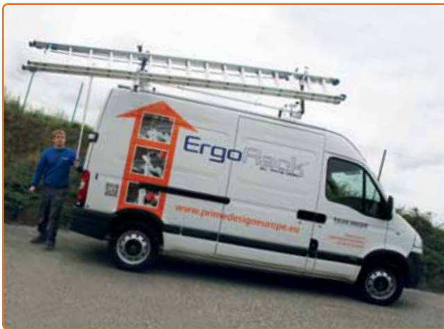
Ergonomic (un)loading of ladders on a vehicle parked on a slope
