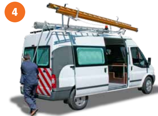
4 - Pull the handle to rotate the ladder onto the roof walking backwards with your arm straight;
